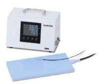
The **TC201** Hemeothermic Blanket System, also called Temperature Controller, is designed to maintain a constant temperature of a subject. The proportional DC power supply slowly varies its output to the heating element based on the resistance of the monitoring thermistor. Electrical noise and switching transients common in AC-based devices is eliminated.
