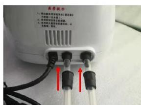
Insert the hoses through the nut and then into the connectors.
