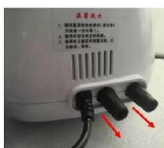
Unscrew the inlet and outlet nuts
